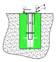
**Step 4:** Securely tighten the screw into place. Before the cement fully solidifies, remove the screw to clean out any cement residue from the hole. Once cleaned, reinsert and tighten the screw securely. Monitor the cement as it sets.
