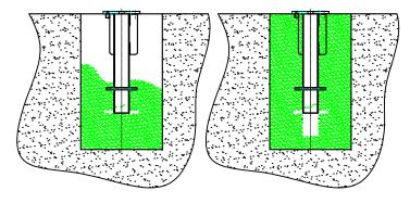
**Step 3:** Align the base so that the metal plate surface is level with the ground. Fill the remaining space around the base with cement until it reaches ground level. Ensure even distribution and compacting. Let the cement cure completely.
