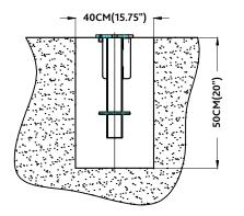
**Step 1:** Select a suitable location for installation. Begin by excavating a hole in the ground with a diameter of approximately 15.75 inches and a depth of about 20 inches.
